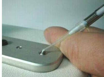
11. Always clean the pedestals after all samples are read and do a measurement with ddH<sub>2</sub>O to be sure you have properly cleaned the instrument.
